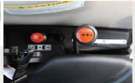
6. 2 range PTO speed to drive commercial grade implements.
